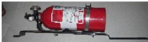
Note: It is a good idea not to mount it to the driver's seat just in case it comes loose and interferes with the pedals – that is the last thing that you want on the track
